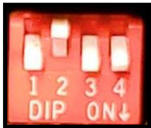
Figure 7 - Dip Switch Setting: "1011" for 24V NiCad
