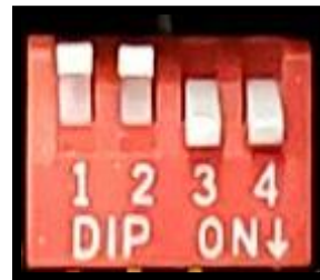
Figure 8 - Dip Switch Setting: "0011" for 12V NiCad
